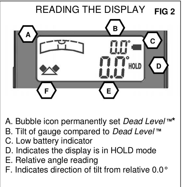
\* *Dead Level™* refers to absolute level with respect to the center of the earth. This is what is shown with a tradition bubble level when the bubble is in the exact center of the vial. Our *Dead Level™* technology consists of a permanently calibrated level setting which is always being displayed by both the bubble level icon and the small digital angle reading in the upper right corner of the display.
