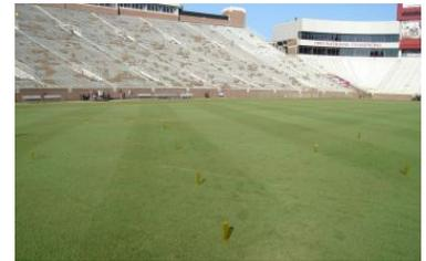
Each set consists of 20 calibrated precipitation gauges that are spread out in a uniform pattern between sprinkler heads. The set consists of 16 large gauges and 4 smaller gauges as well as 20 stainless steel stands for the gauges. They are calibrated in inches and millimeters.
