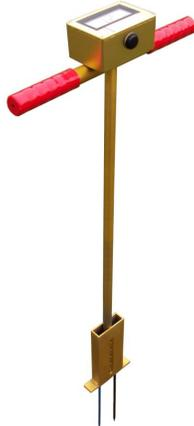
1. Step one, screw in probes- Do not over tighten but be sure probes are very tight.
