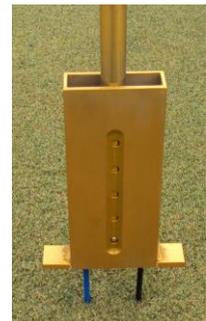
Simply slide the adjustable foot to the desired depth, insert the Turf-Tec Digital Moisture Sensor into the soil and press the "Read" button near the digital display. The read out is
