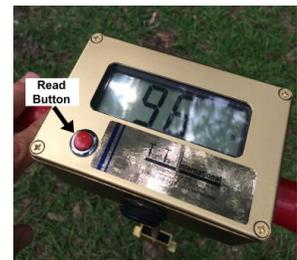
This state of the art unit is designed to work in all soil types and salinity ranges. The probes are also easily replaceable. The Turf-Tec Digital Moisture Sensor uses a newly designed electrical conductivity sensing circuit that gives quick and reliable readings of soil moisture. With years of science behind the sensing results, there is no easier way to test for soil moisture.
