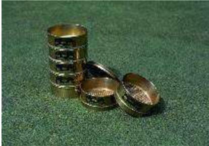
These solid brass sieves are a full eight inches in diameter and are the same type of sieves used by laboratories and Universities for particle size analysis.
