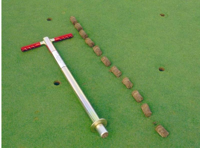
The new Duich Ball Mark Plugger is specially designed for daily removal of ball marks completely out of a golf green and eliminating golfer complaints. The hardened cutter blade removes turf plugs 1-1/2 inches in diameter by 2 1/2 inches deep. The hollow handle fills up with 12 plugs, and the plugs are simply ejected out the top by turning unit upside down.
