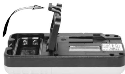
Slide the battery cover (7) in the direction of the arrow and insert new batteries in accordance with the symbols in the battery compartment.
