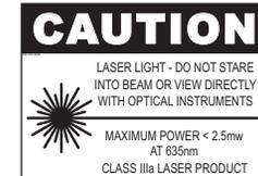
A warning placard is included with each laser and can be attached to the outside of the carrying case. The case can then be placed in a visible location near where the laser is being used in order to meet jobsite posting requirements.
