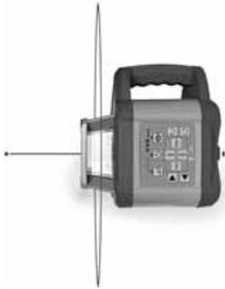
The PLS HVR 505 has third leveling axis (z-axis). Place the instrument as shown. The plumb beam will be leveled automatically. The turning rotor head projects an upright plane to the plumb beam at an angle of 90°. To adjust the alignment line use the arrow keys to move the laser beam right and left.
