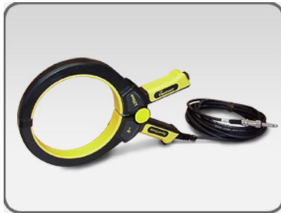
Use the Signal Clamp when direct connection is not possible but you can position a clamp around an accessible target conductor. It applies a relatively stronger signal to the target conductor. The clamp can be used on conductors of 5 inches (12.5 cm) or less in diameter. A threaded fitting on the clamp handle and a remote control jaw actuator are provided for use with an extension handle (hot stick) for long reach applications.
