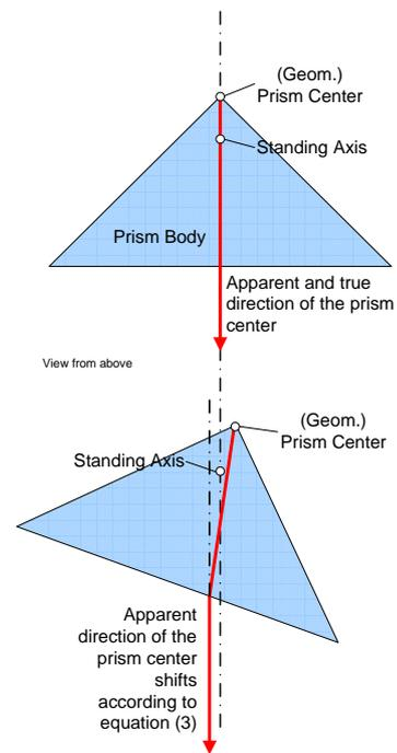
**Figure 18** - True and apparent recognition of prism centers.
