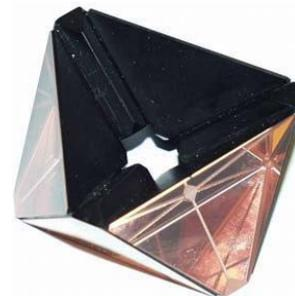
**Figure 5** – Six triple-prism glass assembly.
