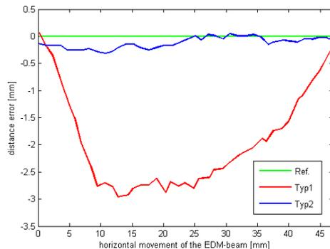
**Figure 14** - Anti-Reflex coating influence on distance measurement.
