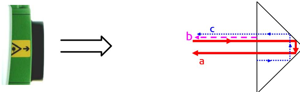
**Figure 12** – Different reflections at the prism caused by the front surface, the inner (front) surface or the 'normal' way through the back surfaces.
