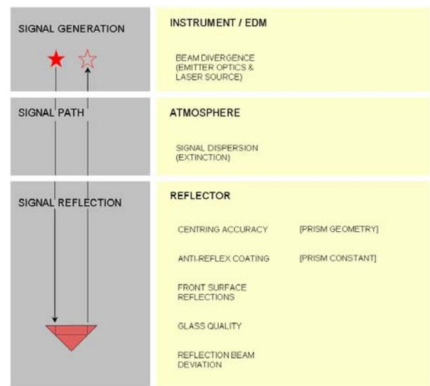
**Figure 1** – Different stages of an electronic distance measurement.
