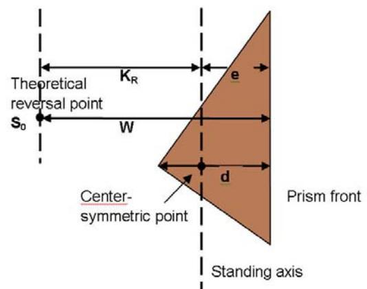
Figure 6 - Cross section through a triple prism.
