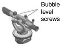
Remove the other half of the error with the two level screws in line with the telescope. If the bubble is still not exactly centered, repeat the procedure. If bubble is off to the right, loosen screw “A” and tighten screw “B”. Otherwise the procedure is identical.
