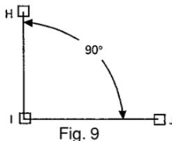
In layout work, it is frequently necessary to set off an angle, usually  $90^\circ$ . Assume that the  $90^\circ$  angle HIJ is to be laid off and points H and I are shown (Fig. 9). Therefore, J is the point you are to set.
