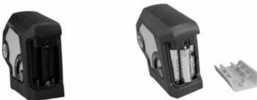
1. As shown in figure, unscrew the battery cover and put 3 “AA” alkaline batteries into the battery compartment noting the polarity as shown in the battery compartment. Screw the battery cover shut. Turn the on/off switch to on. If the power LED is flashing, the battery is low.
