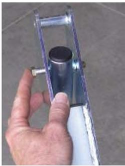
**Step 2:** Start 3/8"-24 self locking nut on to bolt.
