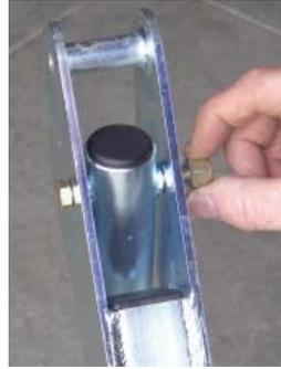
**Step 3:** Swing link arms up to handle. Insert the long 3/8"-24 bolt through link arms and handle. Install flat washer on bolt. Start 3/8"-24 locking nut on bolt.
