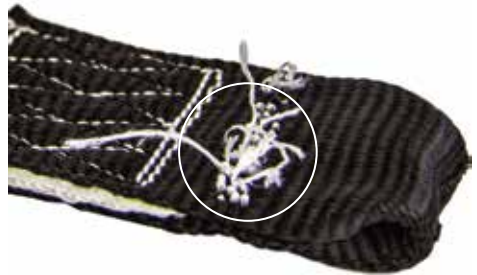
Broken/damaged indicator stitching - Immediately remove from service!
