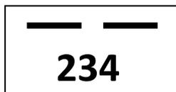
Push the button one time. The bearing is displayed. Use the two linear lines in the display as your aim. Hold the instrument plane when measuring or values may be incorrect! The instrument will compensate the compass angle up to +10 degrees. If leaning the instrument, an image/ message will be displayed urging you to correct the position.
