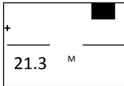
When a result is displayed, aim at the top or other optional height on the same object and press the button again. If you wish to measure more heights on the same object, simply repeat the process of aiming, pressing and releasing the button.
