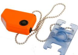
**The HEC-R** offers accurate height results from any known distance. Use the built-in basal area functions to count number of stems in your HEC-R, using one out of four basal area factors (0.5,1,2,4 or 5,10,20,40). The HEC-R will automatically display a calculation of the basal area. One dominant tree height will be used to calculate volume/ha. Measure in m/deg; m/% or ft/deg, ft/% (factory set).
