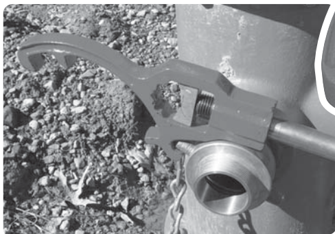
Works on hydrant adapters and hose couplings, both pin and lug type.
