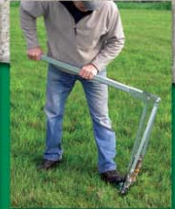
JackJaw® 301 pulling angled stake
