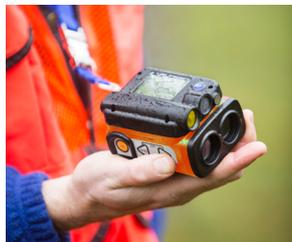
The MD II caliper is adapted for efficient field measurement work. Register diameters, input tree species and send tree heights with IR from the Vertex IV or VL5 instruments. Collect all data in the non-volatile internal memory or transfer online with Bluetooth® to handheld computer, tablet or mobile phone.
