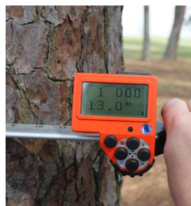
*The MD II computer is rugged and field adapted. Communication and data transfer to external devices is convenient and made with USB cable and Bluetooth®.*
