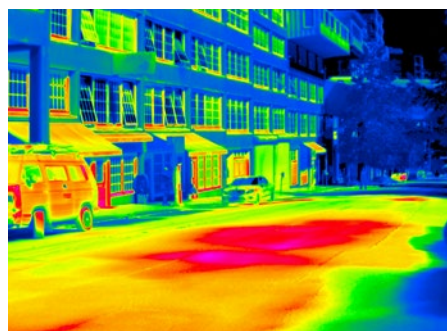
Steam vents under city street
