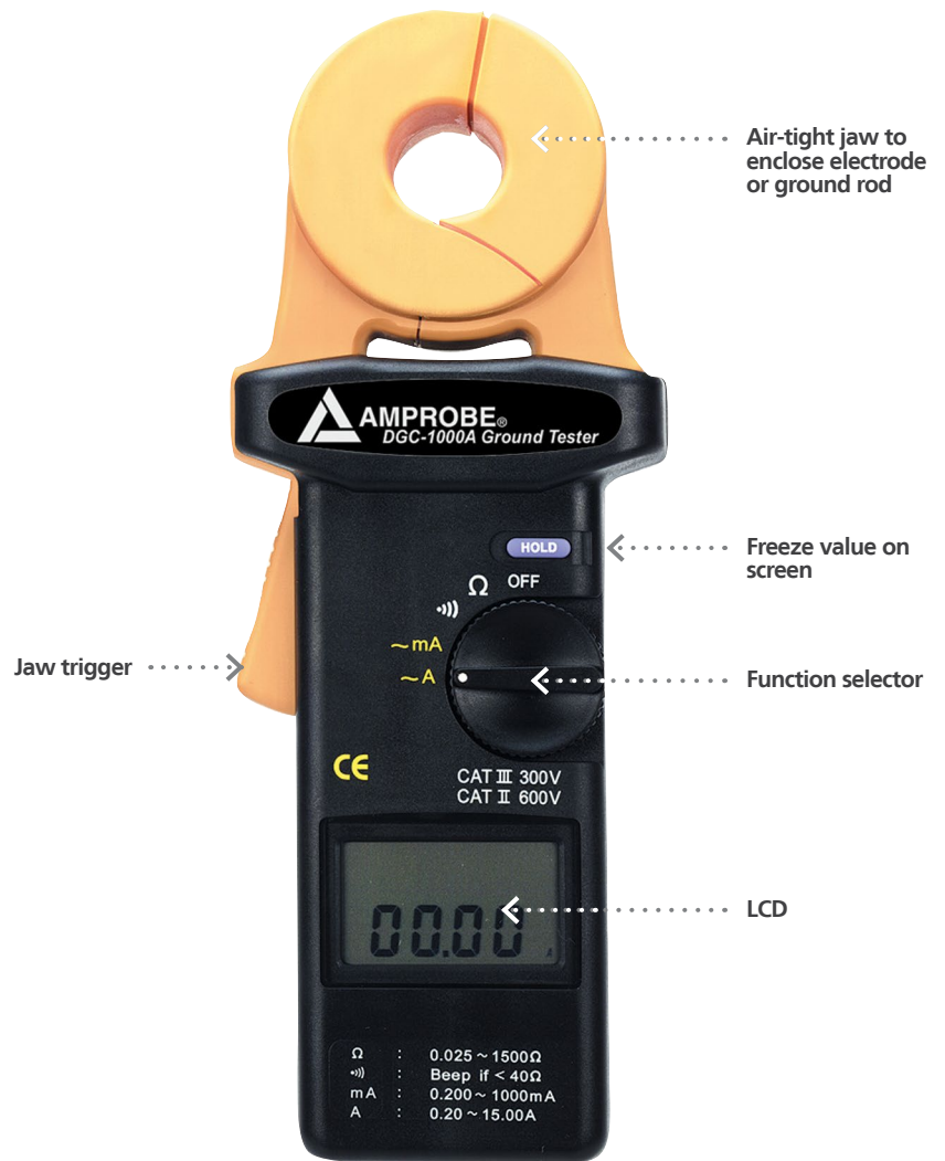
DGC-1000A Clamp Ground Resistance Tester
