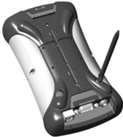
Lock the PowerBoot latches by turning them clockwise one half turn until the arrows on the latches point away from the I/O ports.
